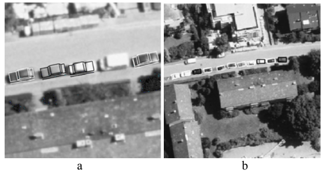
Figure 2. a) Result of the model match. b) Vehicles detected using local model (white) and vehicles recovered through fusion with global model (black)
