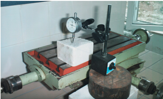
Measurement system by using dial gauge
