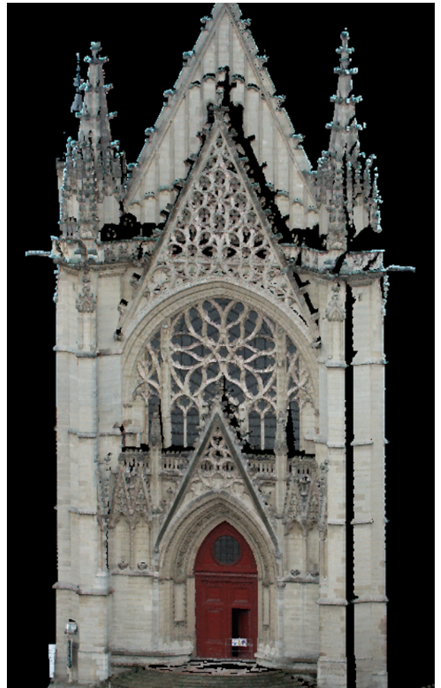
Figure 10: Results on the Vincennes castle chapel. Here, we show the point cloud, where each point has been assigned its image corresponding RGB pixel.
