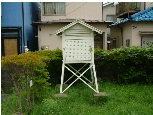
Figure 3. Instrument screen at Kanazawa Nakamura-machi Elementary School (36.56°N, 136.64°E)
