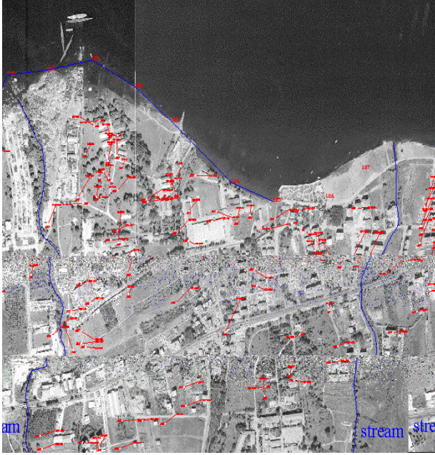
Figure 3. Displacement vectors at Seymen
