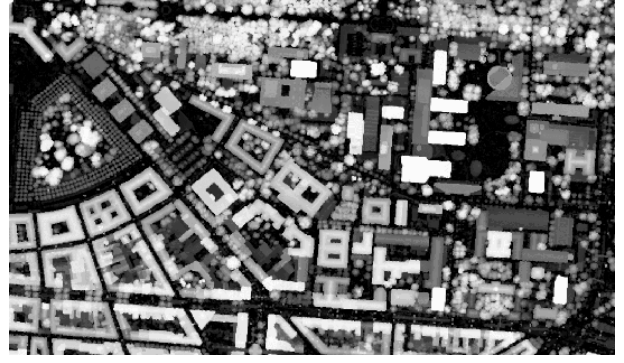
Figure 1: nDSM from laser data (first pulse mode)
