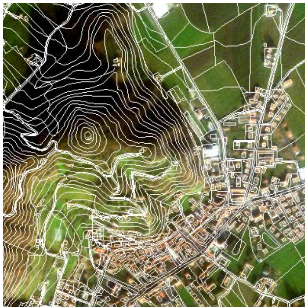
Figure 9 - 1:10000 Vector map overlaid onto the orthoprojected image.
