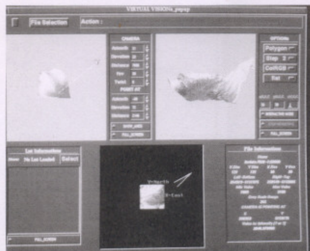
Figure 4 Black and White representation of false colour composite registered and superimposed over DEM using TISS
