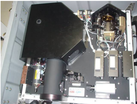
Figure 7. GOSAT FTS bread board model.
