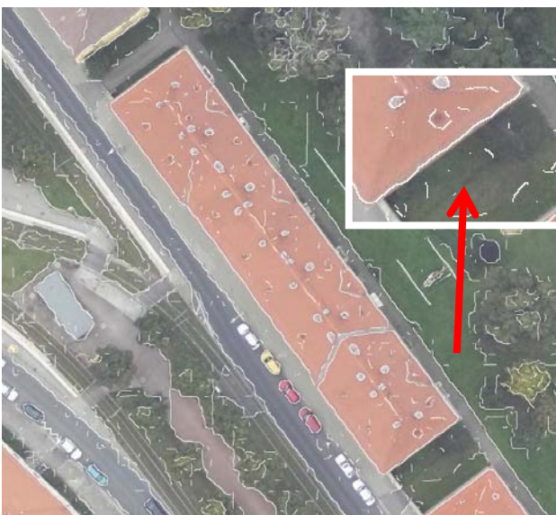
Figure 6. Canny colour edges with shadow-shading
