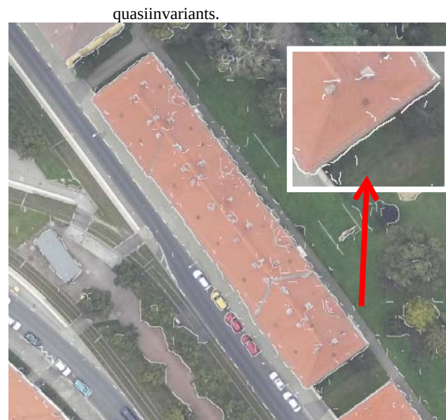
Figure 7. Canny colour edges with shadow-shading-specular quasiinvariants.
